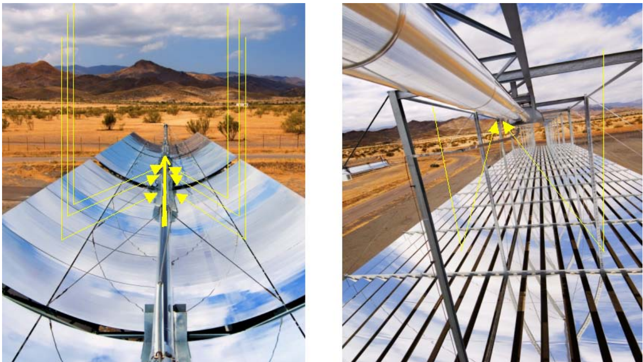
Figure 5.3 Parallel trough and linear Fresnel CSP units showing sunlight focussing on the absorber tube.
