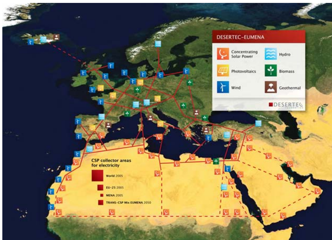
Figure 5.1 DESERTEC EU-MENA Map: Sketch of possible infrastructure for a sustainable supply of power to the EU-MENA region
